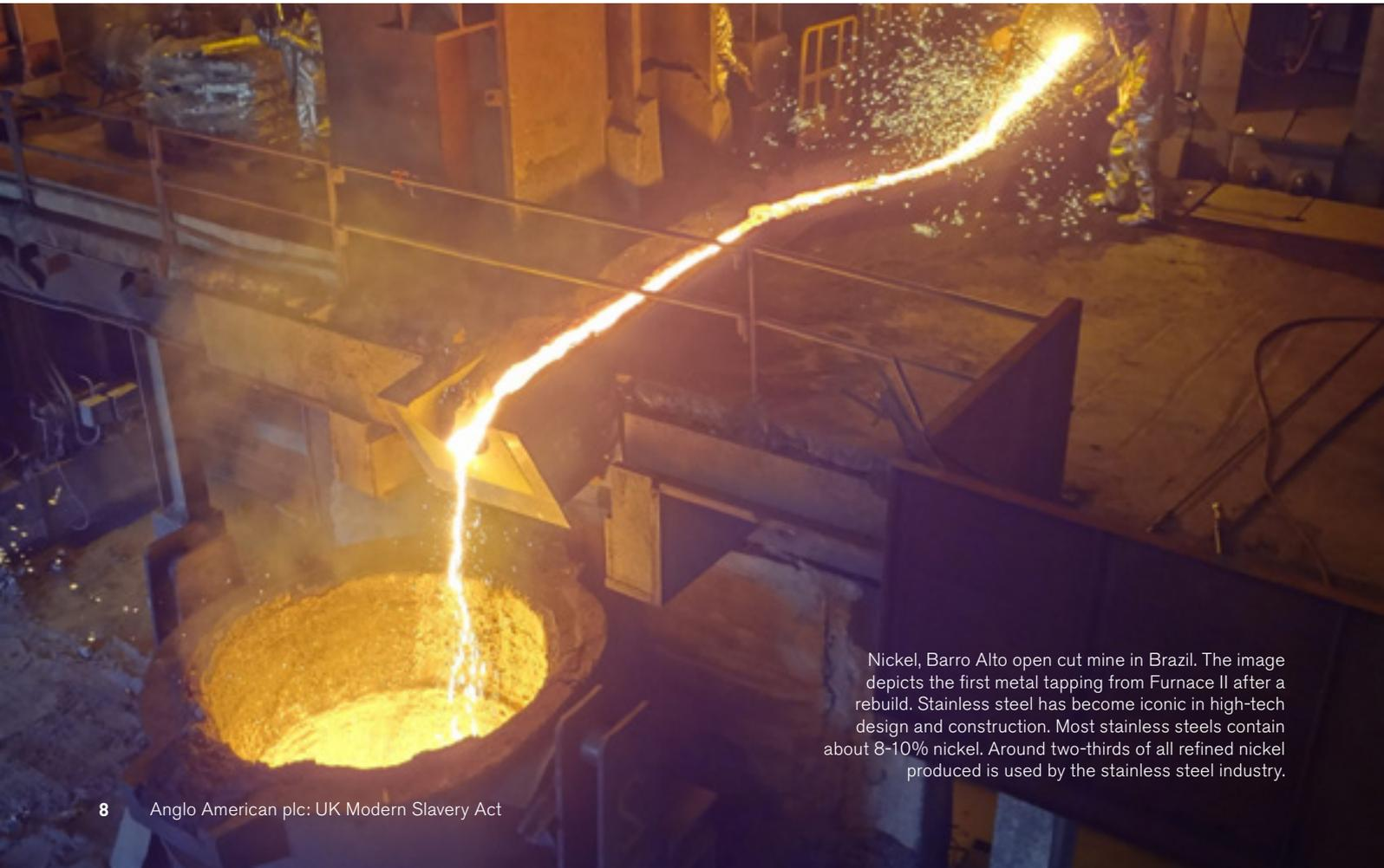
Nickel, Barro Alto open cut mine in Brazil. The image depicts the first metal tapping from Furnace II after a rebuild. Stainless steel has become iconic in high-tech design and construction. Most stainless steels contain about 8-10% nickel. Around two-thirds of all refined nickel produced is used by the stainless steel industry.
